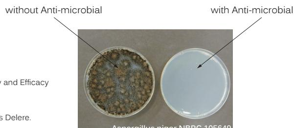
Comparison of growth of bacteria and mold on fan surfaces (microscopic image)
