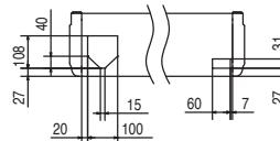
Note) The slope of drain piping inside the unit must take decline of 10mm.
