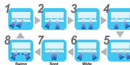
The airflow direction from the right and left louvers can be controlled individually. Eight different air flow patterns can be selected.
