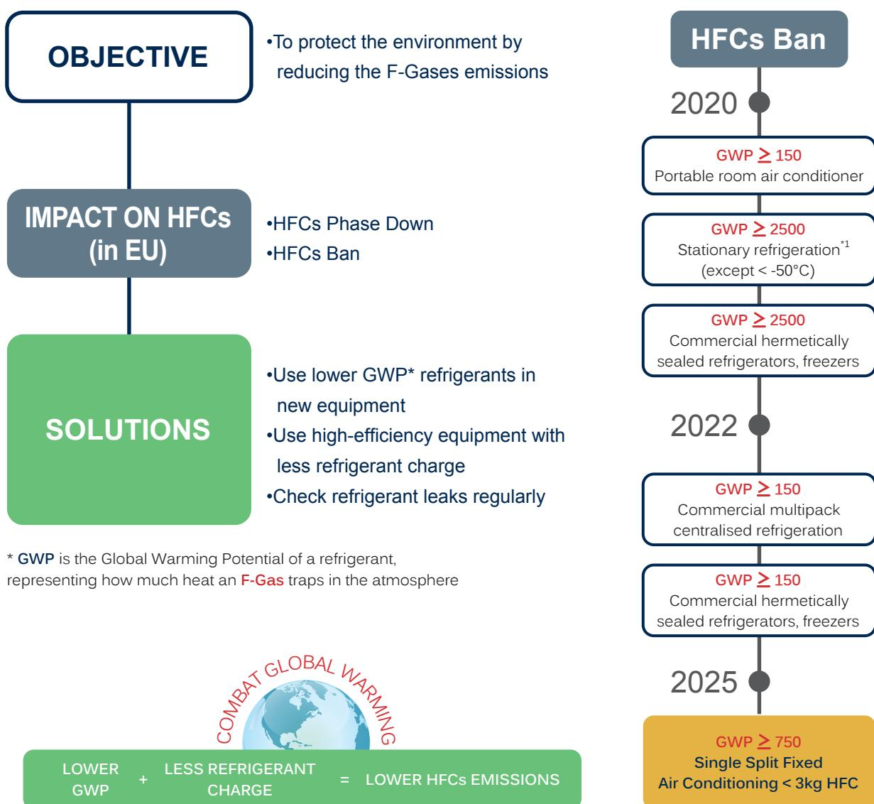
\*1 Stationary refrigeration equipment, that contains or relies its functions upon, HFCs with GWP of 2500 or more except equipment intended for application designed to cool products to temperatures below -50°C application
