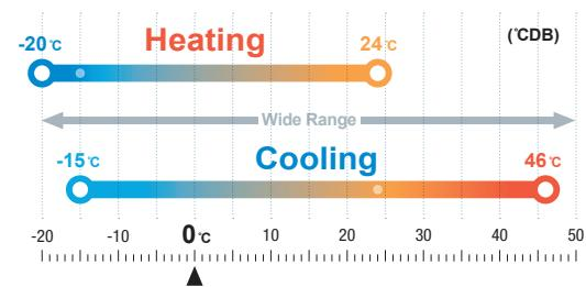
\* For the capacities under low temperature conditions, refer to technical manual.
