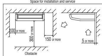
Make a space of 4000 or more between the units when installing more than one.
