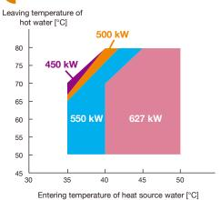
COP Leaving temperature of hot water [°C] 4.5 4.5 5.0 80 3.5 Rated COP achieved 75 6.0 entering temperature of heat source water 70 7.0 45°C and leaving temperature of hot water 80°C. 65 8.0 60 55 50 45
